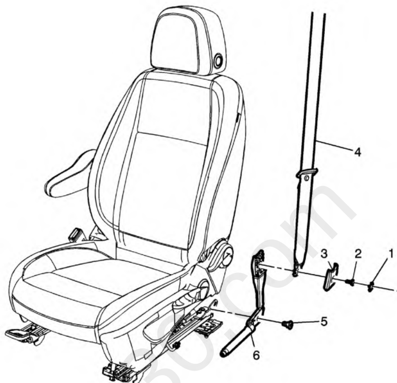
Fig. 48: Front Seat Belt Anchor Plate Tensioner Courtesy of GENERAL MOTORS COMPANY
